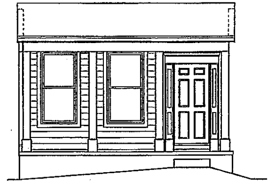
Figure 3.11.2: Porch without railing.
